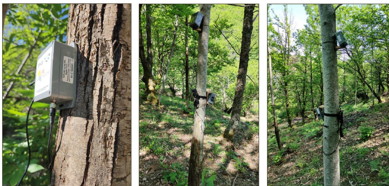
Sensor network in the field: gateway (left), TT+ installed in affected tree (centre) and TT+ installed in healthy tree (right).
