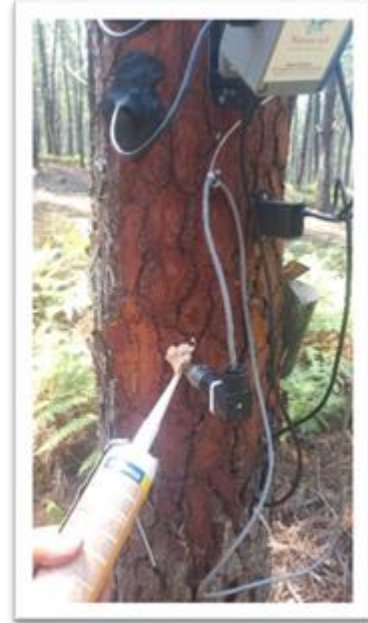
Use of glycerine as transmission vector (left panel) and insulation of the pressure sensor with silicone to prevent air ingress (right panel).
