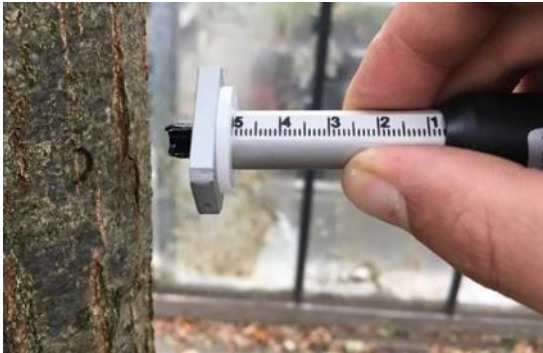
Fig.1: Bark thickness measurement. It is necessary to press the flat tip of the gauge on the bark around the place of installation of the sensor, press the round tip into the bark with the hand. As soon as the tip no longer penetrates the trunk (it has reached the cambium layer), note the bark thickness by looking at the scale and remove the gauge from the trunk.
