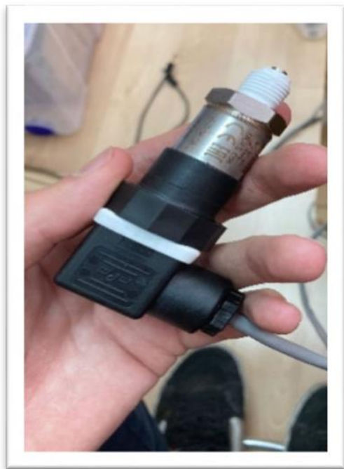
Resin pressure sensor resulting from previous collaborative work between the UPM and the University of Ghent (Belgium).
