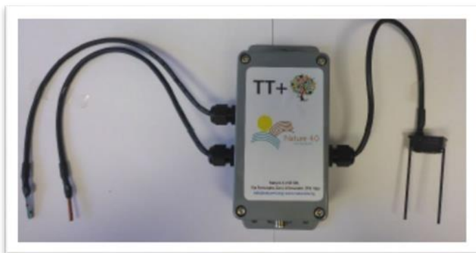
TT-plus with the sap flow and trunk growth probes (bottom), and the resin exudation pressure sensor (right).
