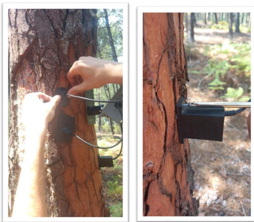
Fig. 2: Detail of sap flow measurement and insulation sensors with Terostat (left panel), detail of dendrometer installation (right panel).
