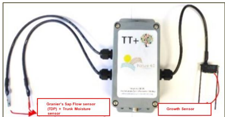
TT+ device in detail. 12- band spectrometre used to assess the canopy evolvement (left), and humidity, sap flow and growth sensor (right).
