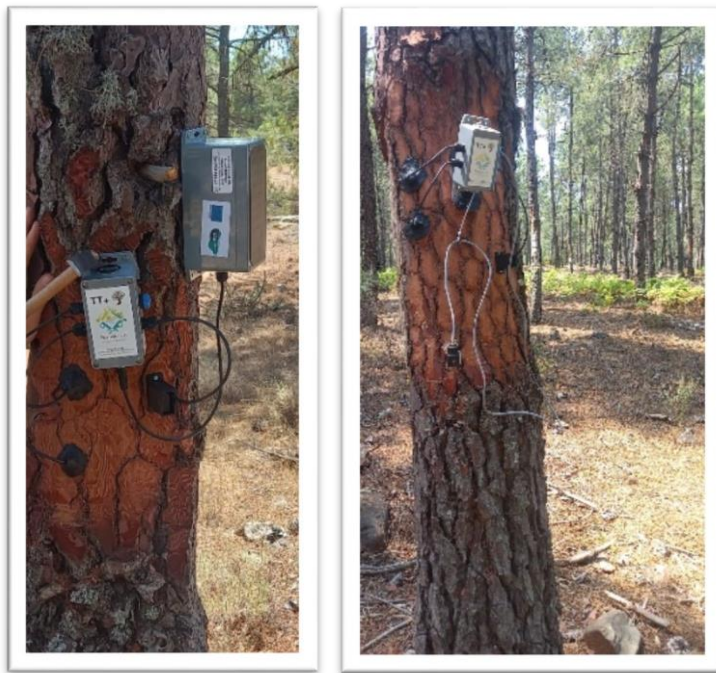
Fig. 3: Installation of a TT-plus with its corresponding battery and probes.
