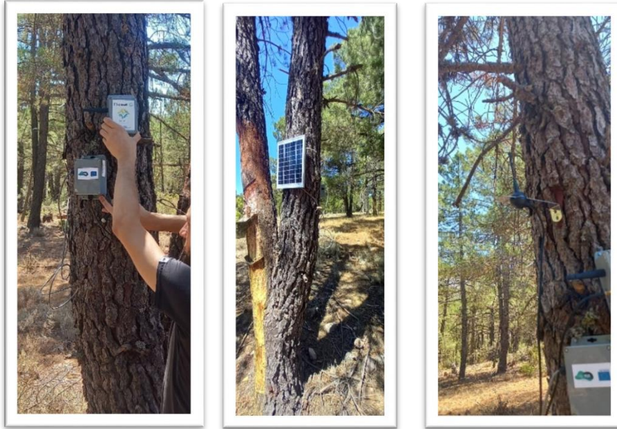
Installation of a TT-cloud and battery (left panel), solar panel connected to the TT-cloud battery (middle panel) and the antennas (right panel). Detail of the two antennas: the grey one is the antenna for sending the signal, the black one (smaller) is the antenna for receiving information from the rest of the sensors.
